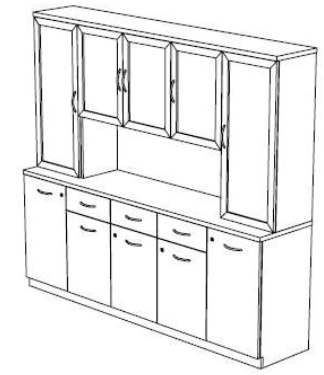
Typical WFN-214 90" Wide Wall 54"W Base with Drawers 2 - 18"W One Dr Base (36"H) 54"W Partial Dr Hutch - Glass Drs 2 - 18"W Full Dr Hutches - Glass Drs
